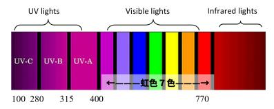
[Ultraviolet rays and UV] The purple range outside of the visible lights in the illustration are the UV lights;
